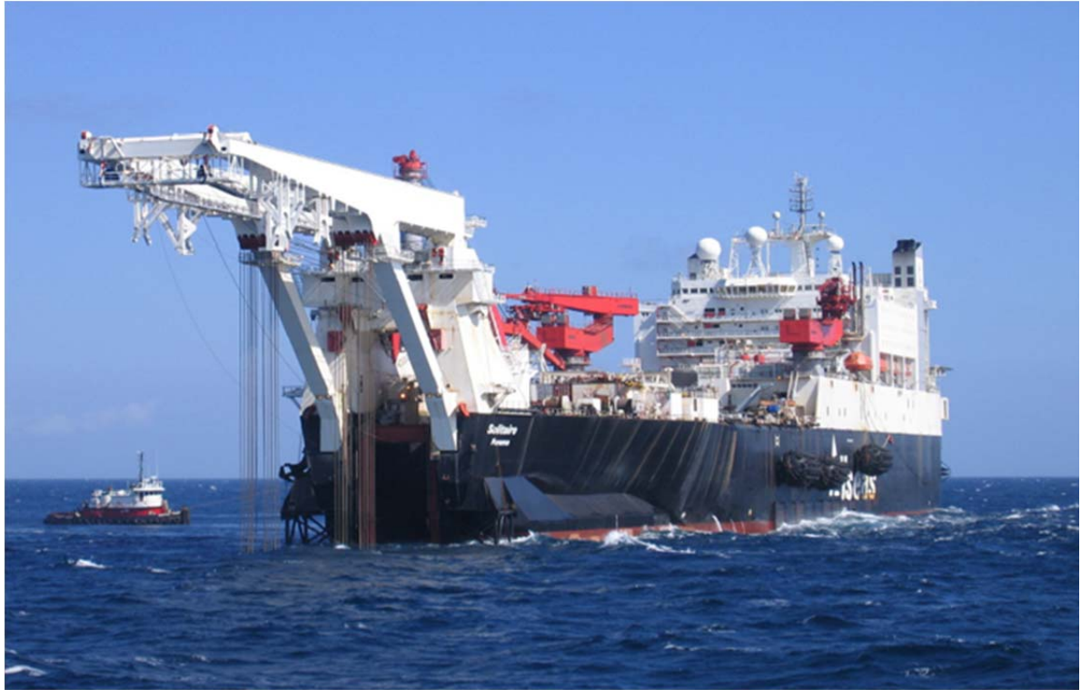
Figure 2.14: The 4th Generation Dynamically Positioned Pipelay Vessel “Solitaire”
