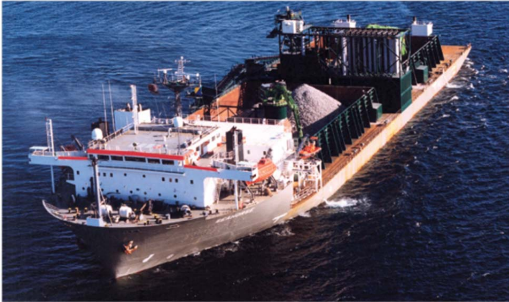
Figure 2.26: Example of Fall Pipe Rock Dump Vessel
