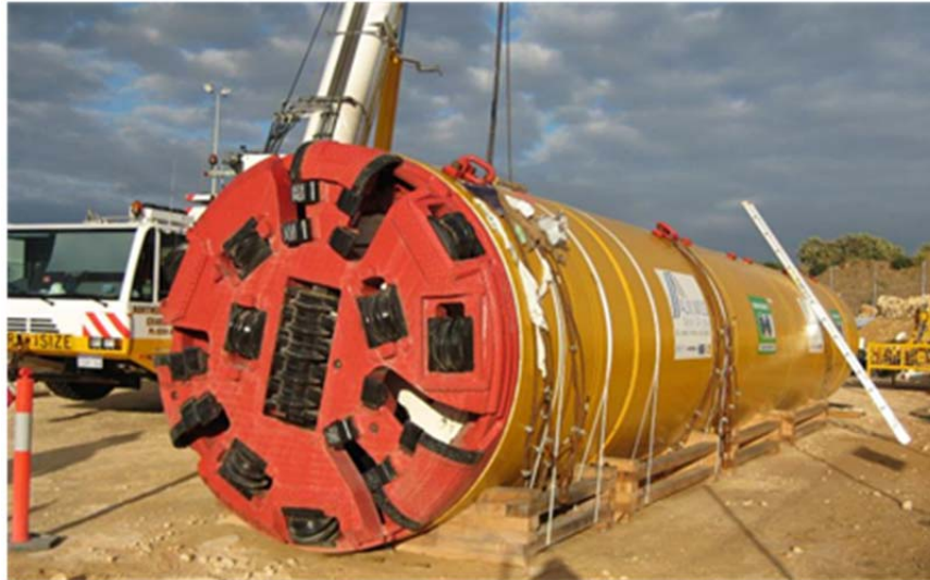
Figure 2.4: Example of a Tunnel Boring Machine
