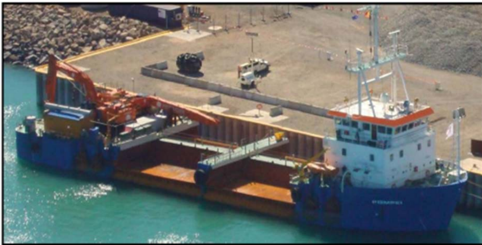
Figure 2.24: Example of a Side Stone Dumping Vessel
