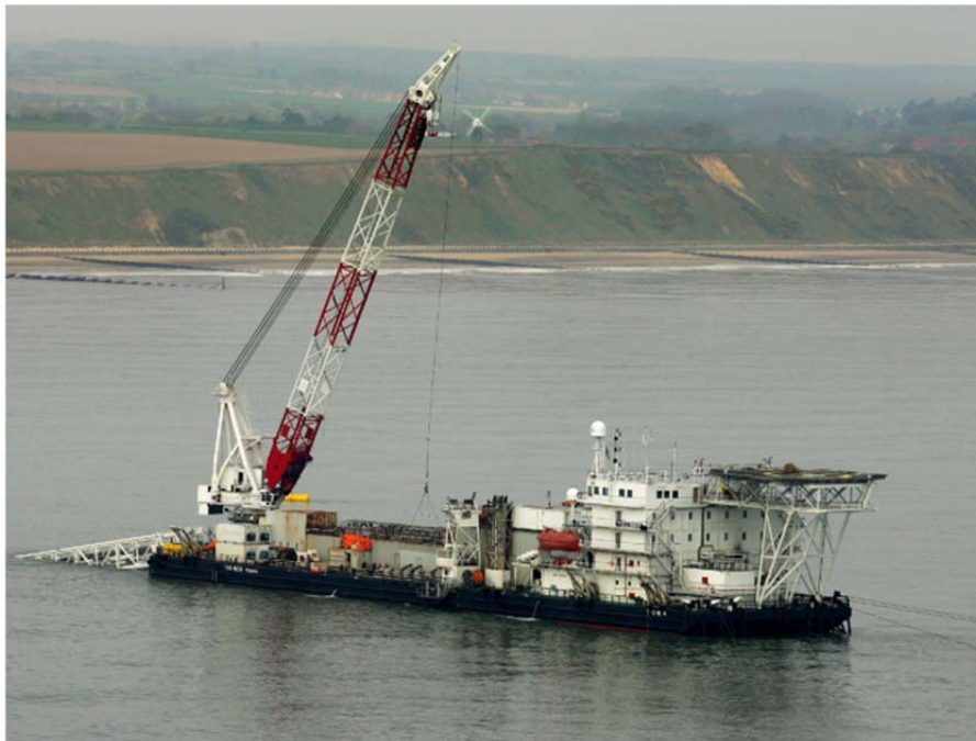
Figure 2.15: The 2nd Generation Moored Lay Barge “TogMor”
