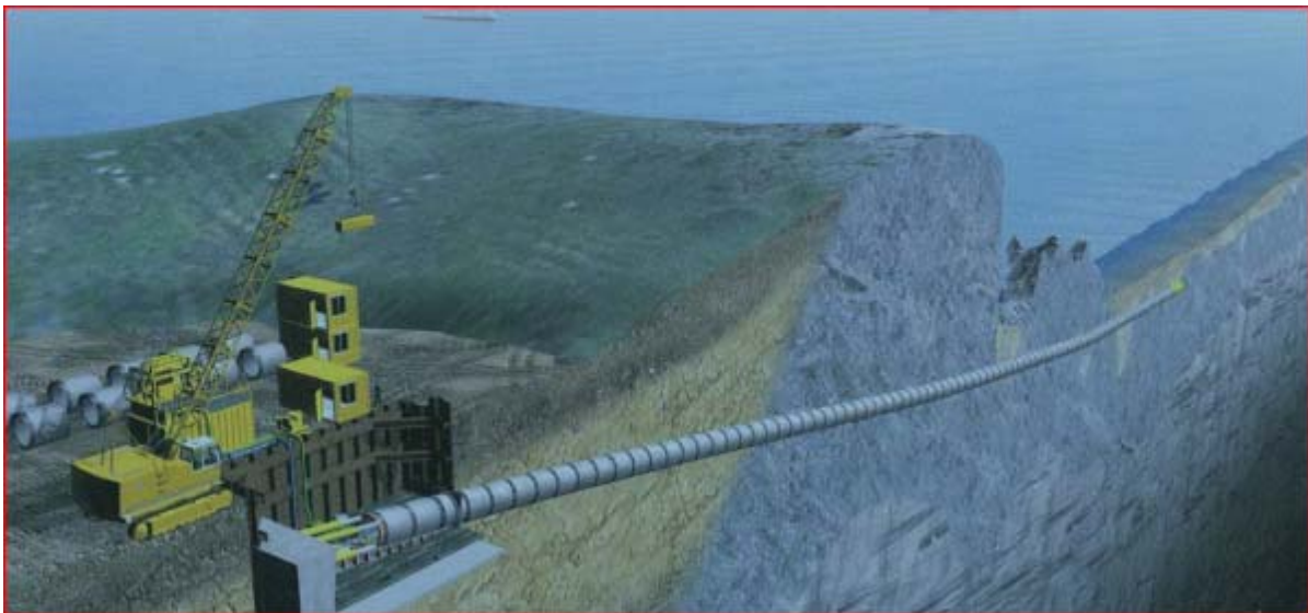
Figure 2.2: Schematic of the Microtunnel
