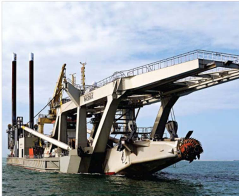
Figure 2.9: Typical Cutter Suction Dredge
