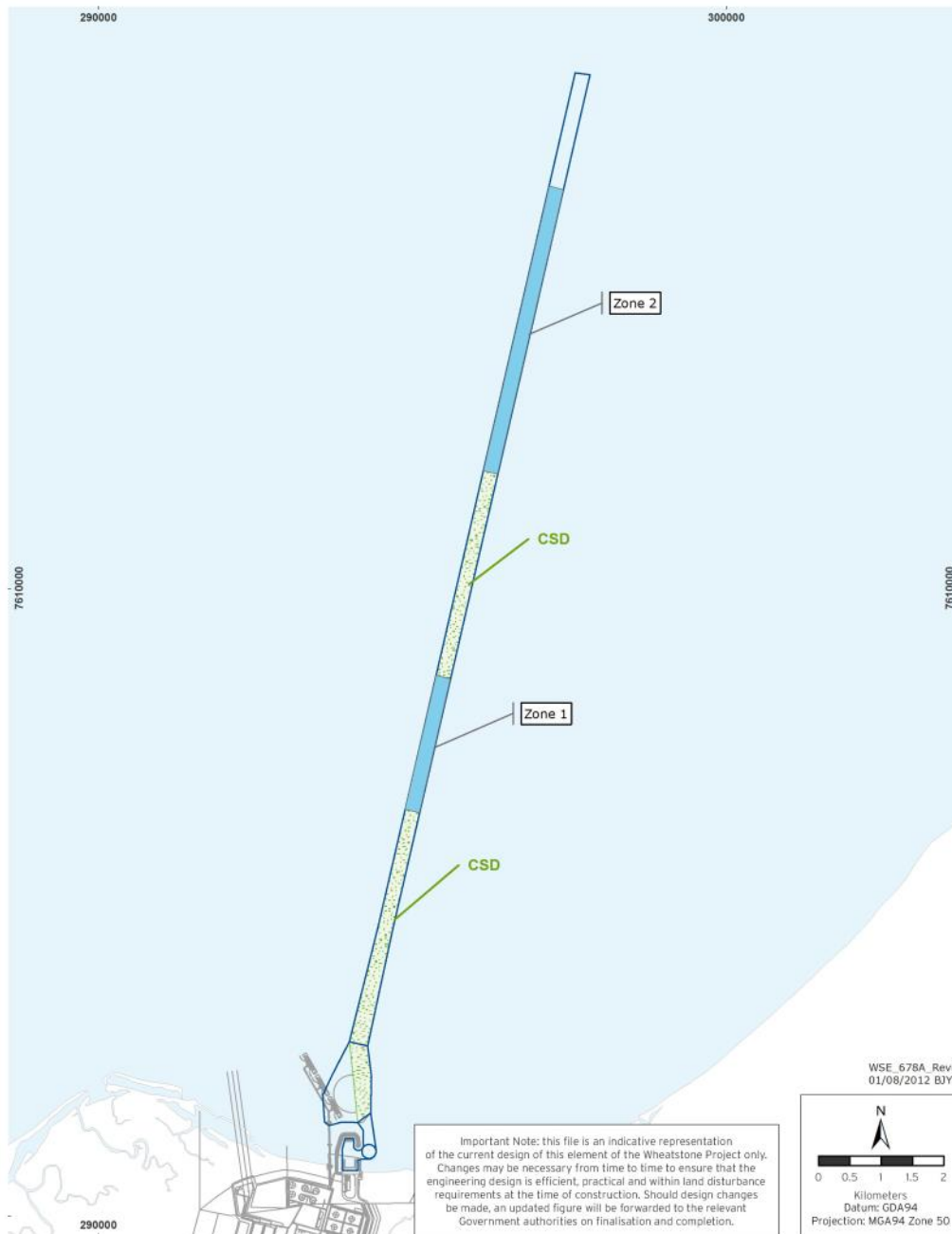
Figure 2.14: CSD Dredging Approach Channel
