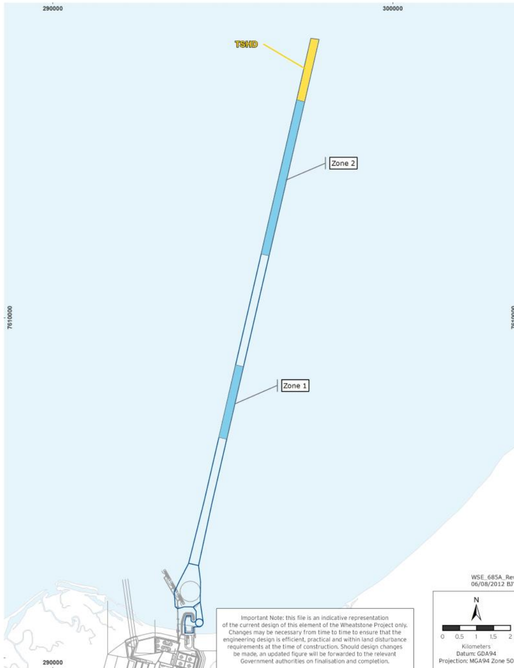
Figure 2.15: TSHD Dredging northern part of Approach Channel
