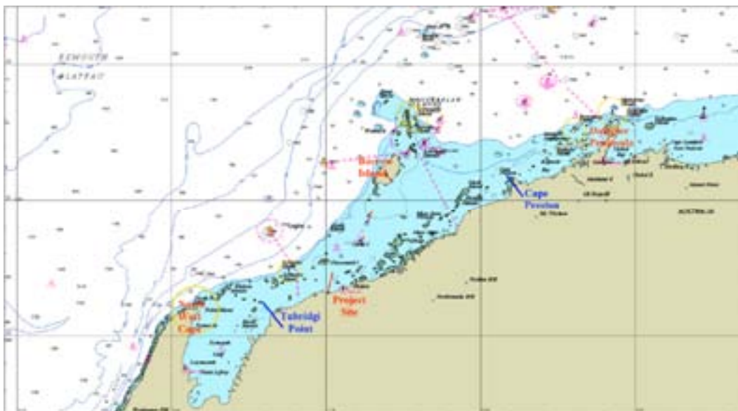
Figure 2.5 Sketch of project site along North-northwest facing section of Pilbara Coastline. Light blue coloration indicates depths less than 30m CD. Green areas indicate reefs and rocks drying out at low tide.
