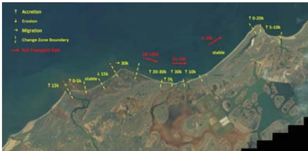
Figure 5-13: Erosion, Accretion and Net Transport Rates Derived from aerial photos 1963-2009 1 . Quantities are m 3 /yr.
