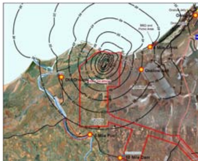
Noise Contours for Normal Plant Operation
