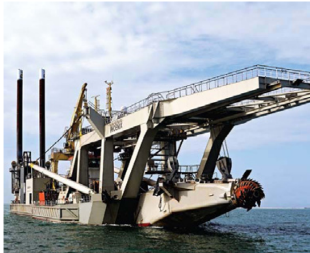
Figure 4-6: Example of Cutter Suction Dredge (CSD)
