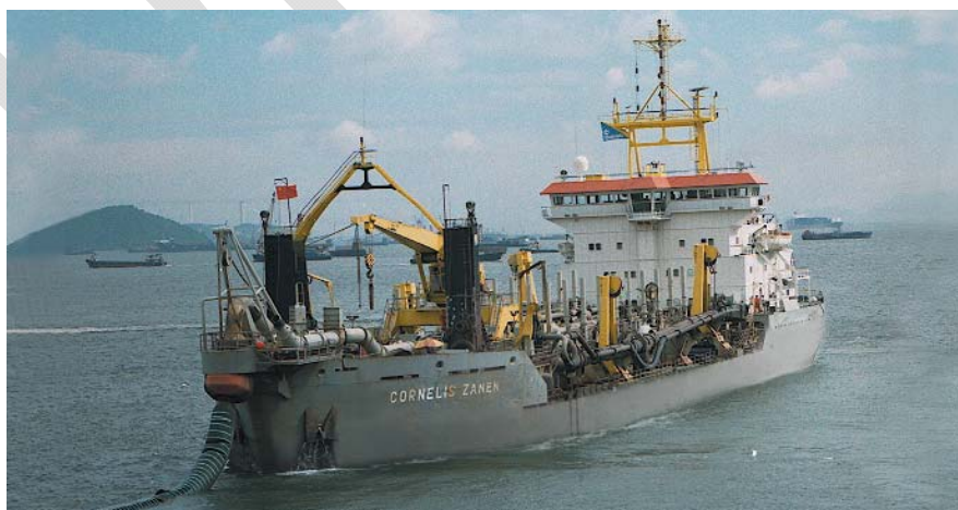
Figure 4-8: Example of Trailing Suction Hopper Dredge (TSHD)
