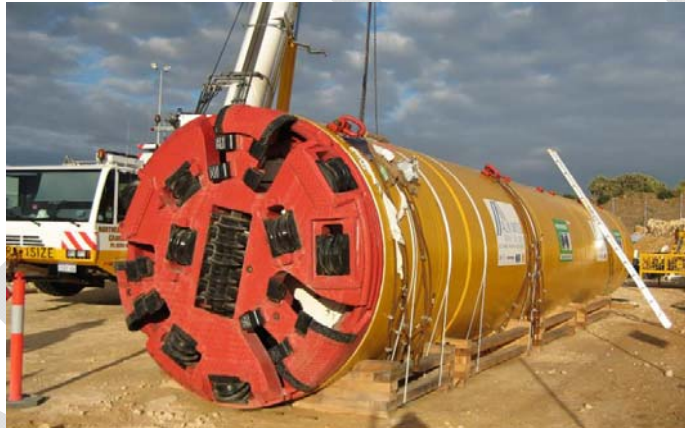
Figure 4-7: Example of a Tunnel Boring Machine (TBM)
