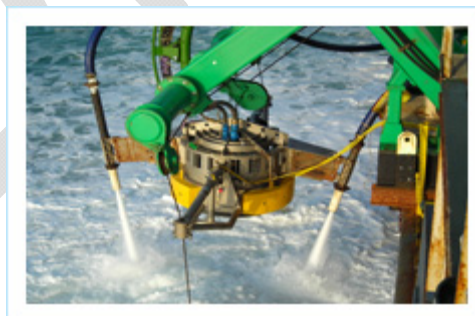
Figure 4-11: Example of a Mass Flow Excavator
