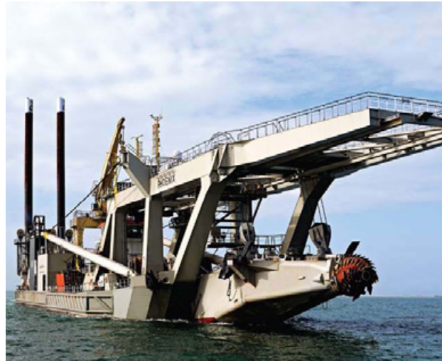
Figure 4-9: Example of Cutter Suction Dredge (CSD)
