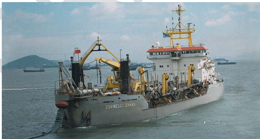
Figure 4-5: Example of Trailing Suction Hopper Dredge (TSHD)
