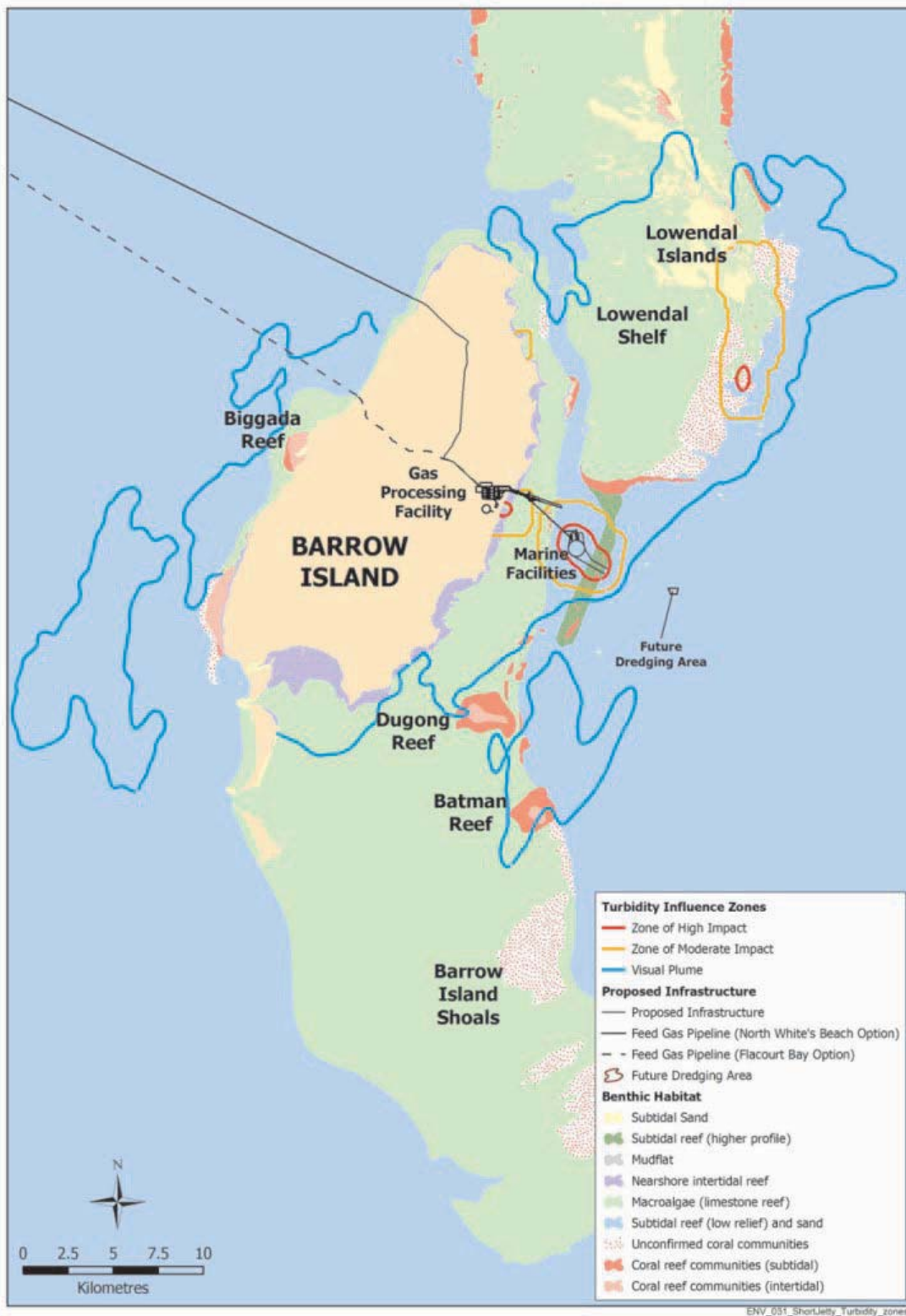
Figure 7.6 Mortality zones derived from TSS data for the “Base” case with the UKC of the THSD controlled to 4 metres. Level 1 (red) = high impact, Level 2 (orange) = moderate impact, Level 3 (blue) = visible plume (exposure above 2mg/litre)..
