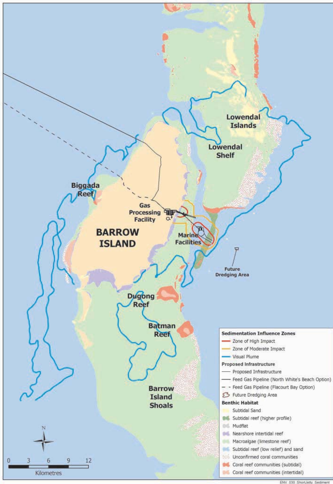
Figure 7.5 Mortality zones derived from sedimentation data for the “Base” case with the UKC of the THSD controlled to 4 metres. Level 1 (red) = high impact, Level 2 (orange) = moderate impact, Level 3 (blue) = extent of sedimentation (1 mg/cm 2 ).
