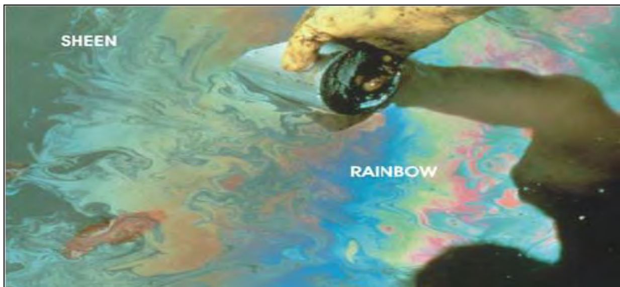
Figure 2-10: Photographs of oil film appearance on the water surface. Top panel indicates bands of dull metallic colour surrounded by rainbow and silver sheen. Lower panel indicates Rainbow sheen thinning to silver sheen (Source: "Oil on water sheens" – Ron Goodman Innovative Ventures Ltd).
