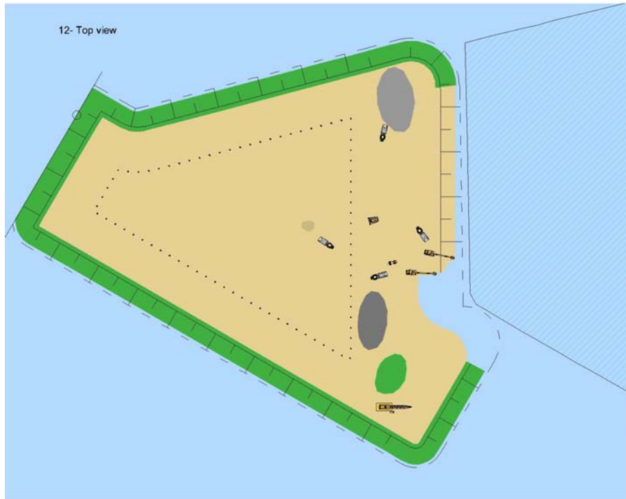
MOF area is prepared for the installation of the abutment structures. Armour material, along with fill material, is stockpiled on the MOF area.
