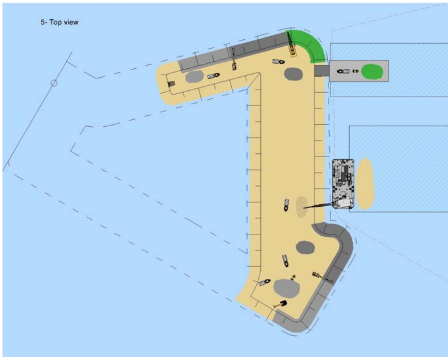
Dredged material continues to be rehandled ashore for use in the construction of the MOF bunds in conjunction with the placement of armour materials.
