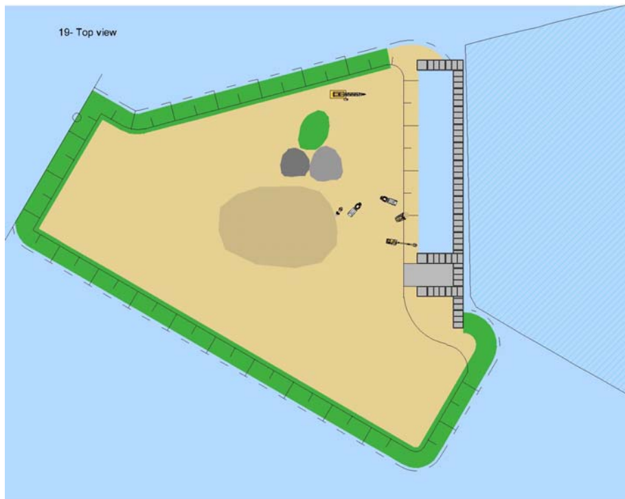
Fill material, which has previously been stockpiled on the MOF, is then placed behind the caissons.
