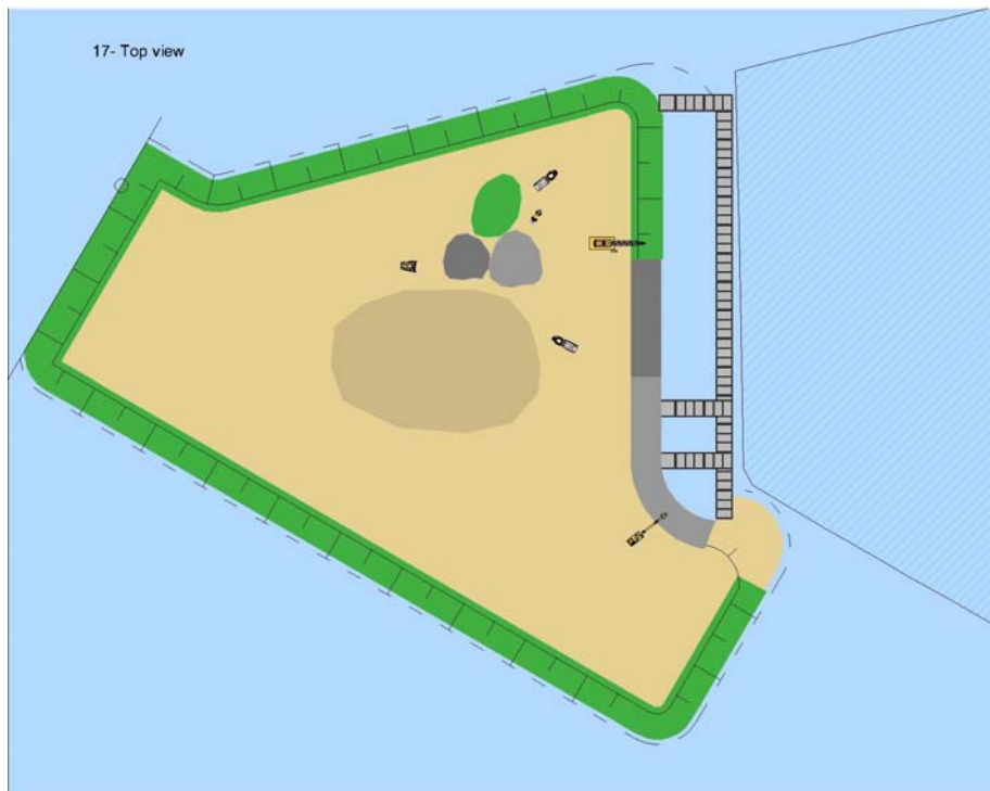
Once caissons are in place, armour materials from behind can be removed and stockpiled on the MOF.
