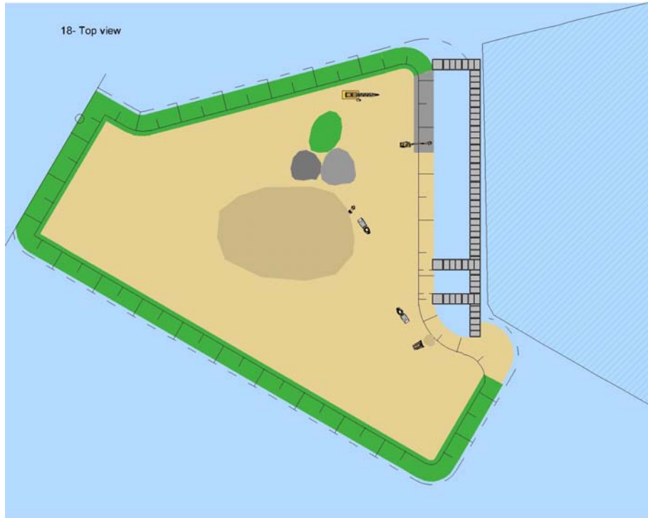
Armour material from behind caissons continues to be removed.
