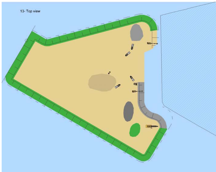
Once trimmed to the correct profile, armour material will again be placed for protection.
