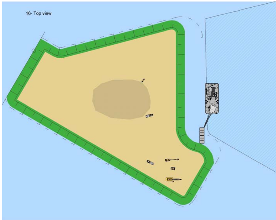
Upon completion of the armouring works, a crane barge is used to place the abutment caissons.
