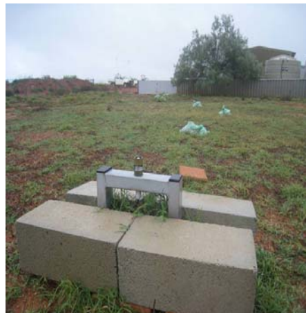
Plate 13-1 Terrestrial Light Sensor and Data Logger Deployed during the Marine Baseline Program for the MOF and LNG Jetty
