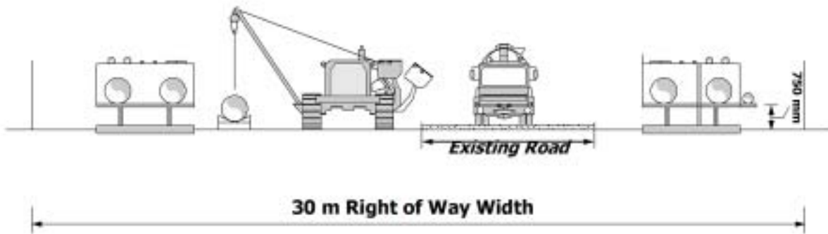
Figure 6-15: Pipeline Installation Technique
