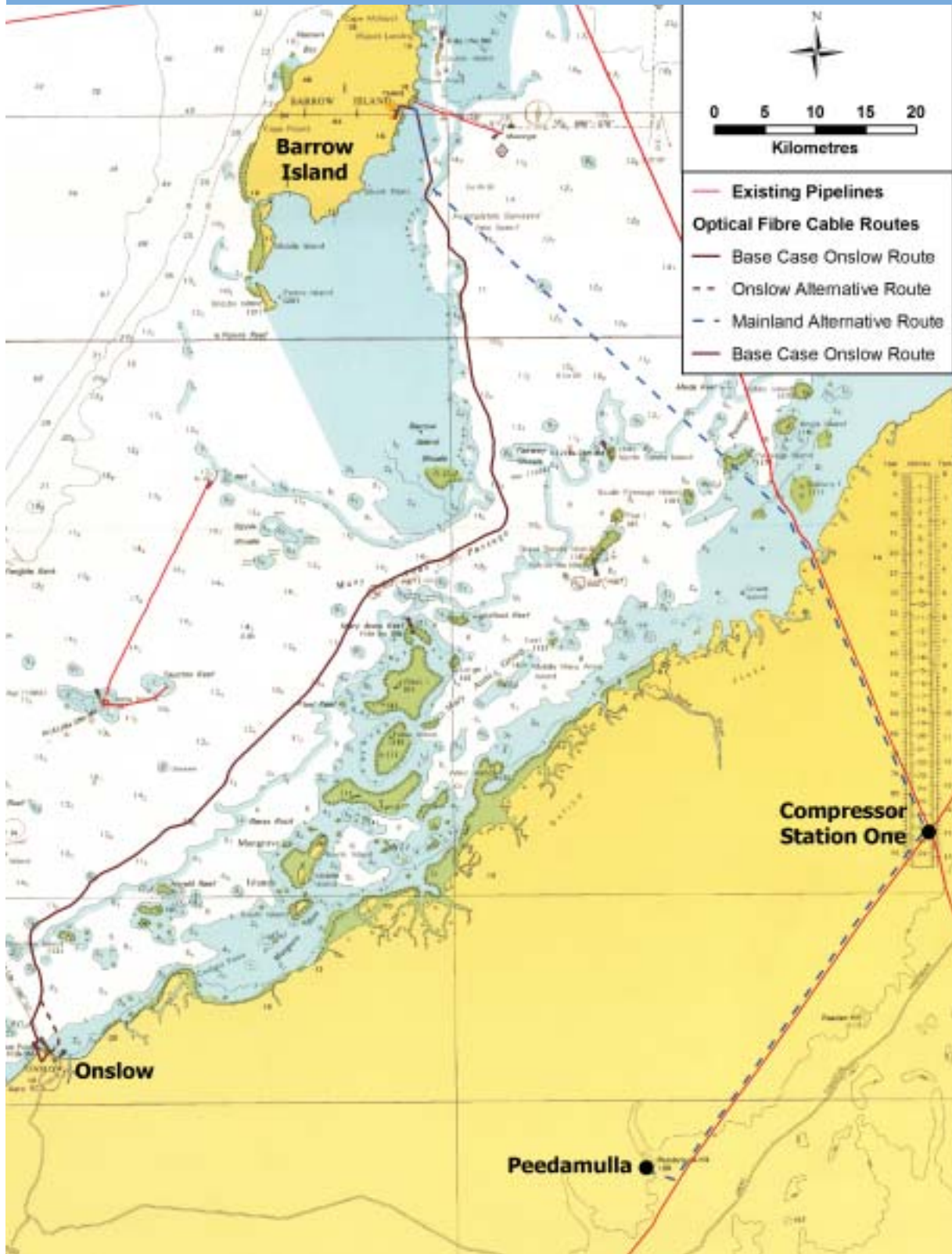
Figure 6-3: Possible Routes for Optical Fibre Communications Link
